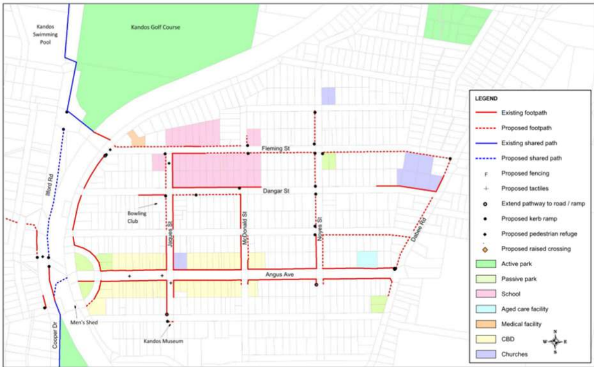
Figure 4: Kandos Footpaths as shown in the PAMP with proposed footpath and kerb ramp in front of the Museum frontage on Buchanan Street.
